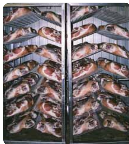
Smoke-trolleys with angle-grids for ham
